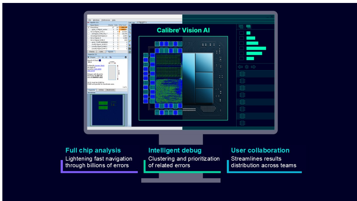
Figure 2. The Calibre Vision AI tool speeds up full-chip physical verification with intuitive navigation, intelligent error clustering, and collaborative results sharing—making debug and signoff faster for everyone involved.
